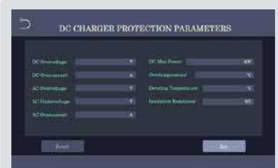
Screen for setting HVDC output protection parameters.Voltage, current, power and temperature protection parameter setting
